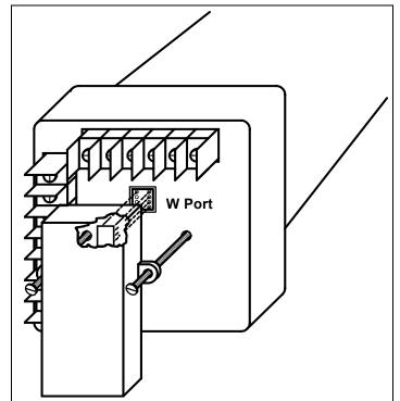
**Diagram 2.4**: Optional Communication Converter or DC Output Module Installation \* Recommended wire gauge is 20 AWG for DC Output or RS-485 options.
